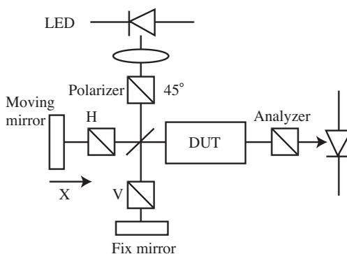
Figure 7. Interferometric working principle
