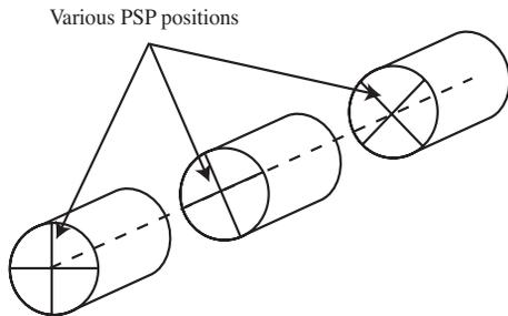
Figure 4. Transmission fiber model with 3 birefringence sections with different orientations of input PSP and birefringence values
