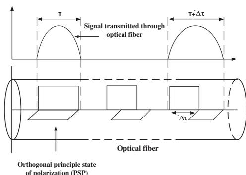
**Figure 2. Effect of DGD to signal propagation in birefringence fiber that results in pulse spread**
