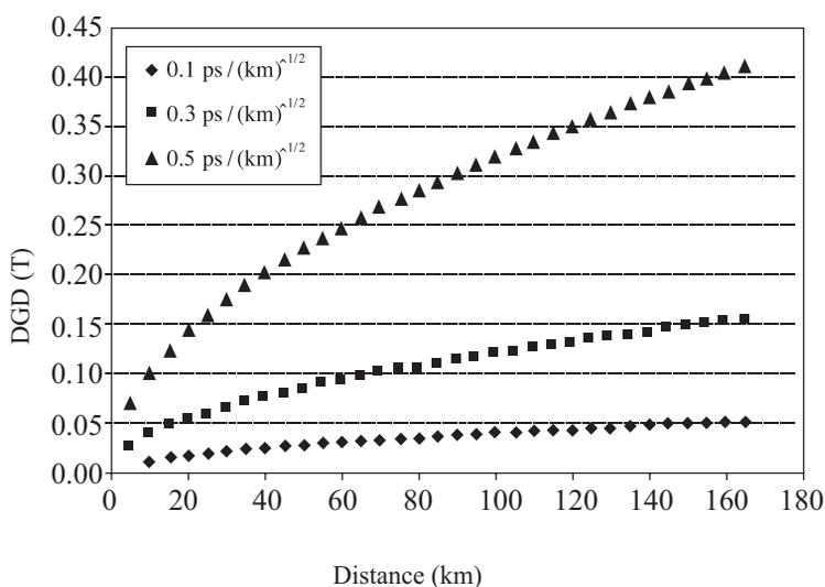
Figure 10. DGD (T) vs distance (km) for fiber with several PMD coefficients at 40 Gbp rate
