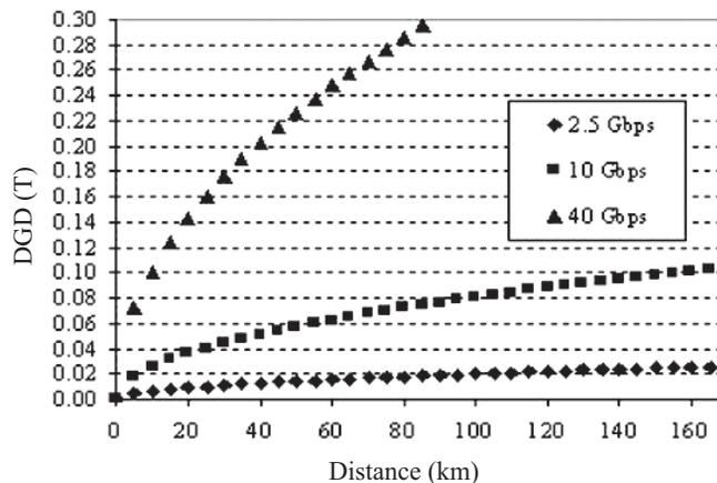
Figure 11. DGD (T) vs distance (km) for several bit rate by using  $0.5 \text{ ps}/(\text{km})^{1/2}$  PMD coefficient fiber
