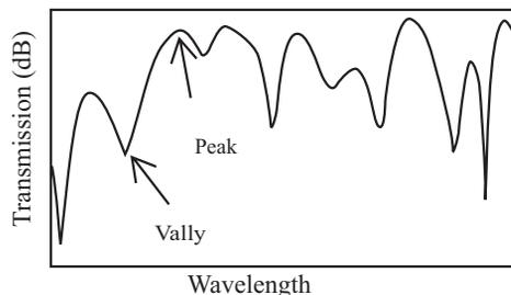
Figure 5. A typical Fixed Analyzer measurement result (Francia *et al.*, 1998)
