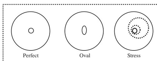
**Figure 1. The mechanical stress due to movement of the fiber resulting in a dynamic aspect to PMD**
