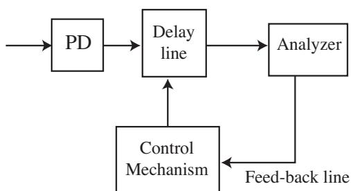
Figure 9. Block diagram of OPMDC, PD: Photodetector
