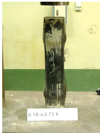
Figure 9. Typical modes of failure of the test specimens (a) RC column, (b) and (c) tubed RC columns with t = 3.2 and 4.5 mm, respectively
