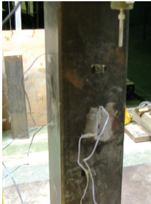
Figure 5. Strain gage installation at the mid-height of a tubed RC column specimen
