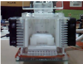
Figure 2. Thermoelectric temperature control box with a cooling fan on each active thermoelectric module. (a) front view, (b) top view, (c) front view with QCM cell inside
