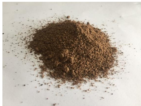
Figure 1. Photos of palm oil residue for preparation of biocoke
