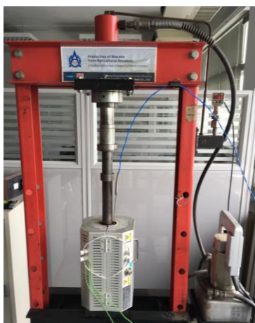
Figure 2. Photo of the apparatus for preparation of biocoke
